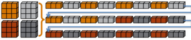
Figure 7: Flattening a 2D distributed array. The block owned by a process becomes discontinuous when representing the 2D array in 1 dimension.
